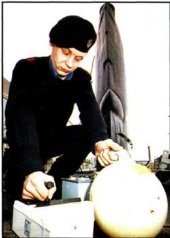
Emphasis on safety. . . A rating monitors hull radiation levels on a nuclear powered submarine.
