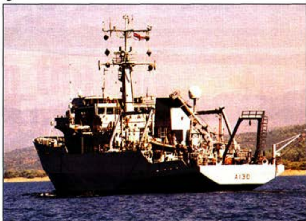
• ABOVE: HMS Roebuck, in her new grey livery, operates within 400m of shore using her towed sonar. • LEFT: AB(SR) Christopher Hadlow makes a splash by surveying the beach gradient in the Greek surf.
