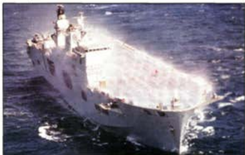
● HMS Ocean tests her pre-wetting system en route to the Arabian Sea.
