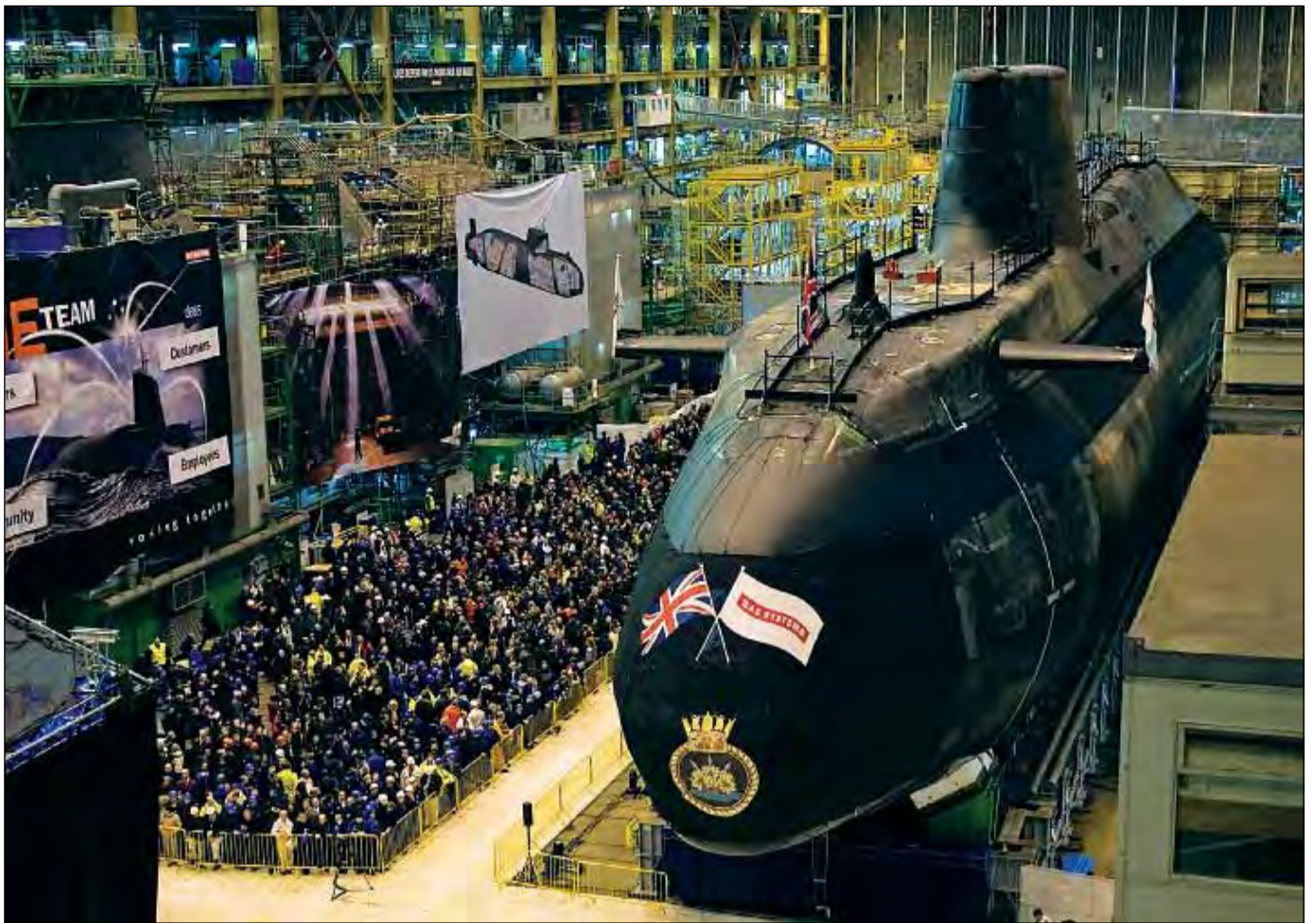
Thanks to a giant synchro-lift the 7,400-tonne £1bn boat was lowered gently into the water in the early part of January, then moved into the adjacent dock where she will remain firmly secured while the next battery of tests is carried
