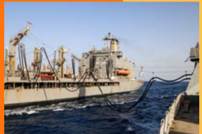
HMS Diamond (right) conducting a replenishment at sea (RAS) with USNS Kanawha - a welcome top up of supplies Image by: LPhot Chris Sellars
